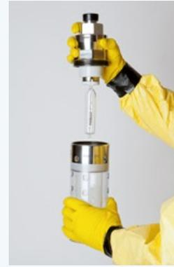
The BIRNS Curie connector does not depend on the rubber-coated pin method of sealing, as seen in other competitors units. Instead, it has redundant captivated o-ring seals in stainless steel grooves, to preclude any possibility of electrical leakage.
