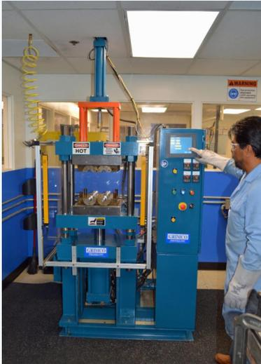
We recently enhanced our existing molding capabilities with the addition of a new custom 40 ton hydraulic transfer press. It will provide additional firepower to BIRNS' molding facility for connector inserts, allowing computer controlled precision for functions like injecting glass reinforced epoxy (GRE) and providing increased speed and output for large orders.
